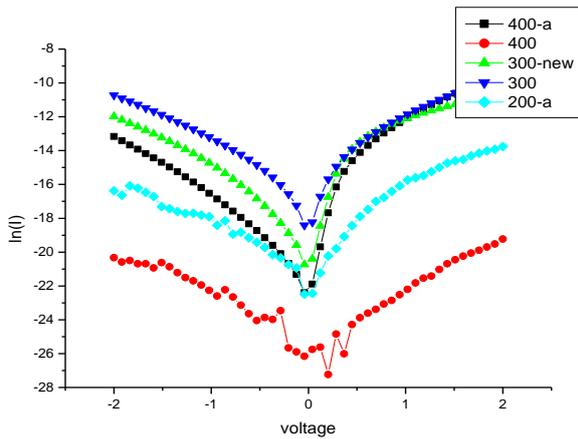
Fig 3: I-V characteristics for different annealing temperatures
