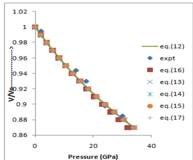
Figure1:Pressure dependence of  $\frac{V}{V_0}$  for nanocrystalline nickel(20nm)
