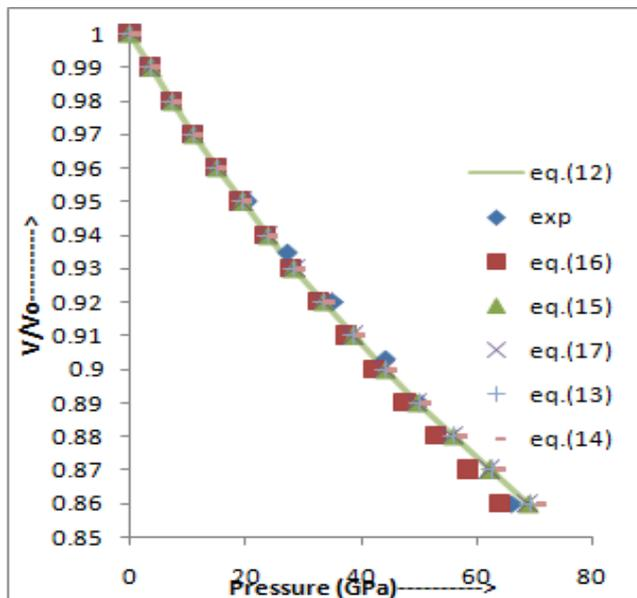
Figure 4: Pressure dependence of  $\frac{V}{V_0}$  for  $\gamma\text{-Si}_3\text{N}_4$
