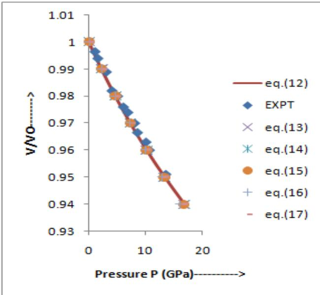
Figure 2: Pressure dependence of  $\frac{V}{V_0}$  for  $\text{TiO}_2$  (rutile phase)
