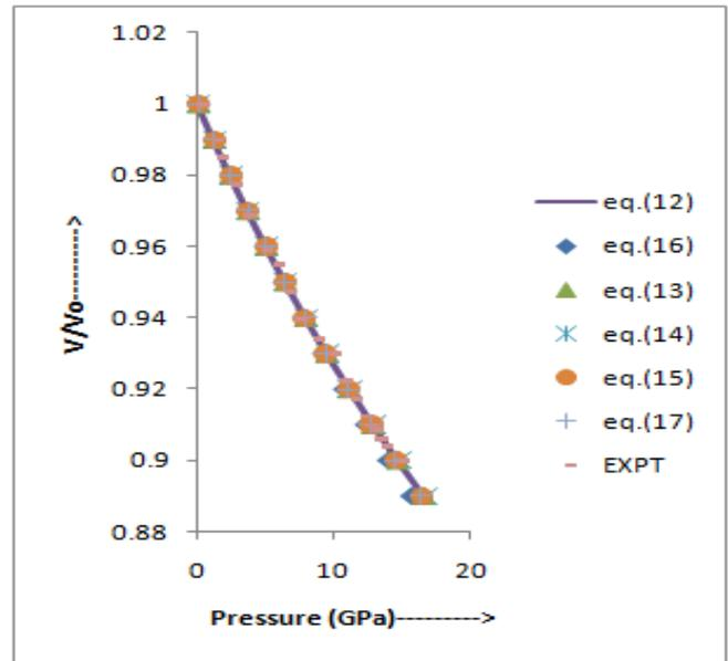
Figure 5: Pressure dependence of  $\frac{V}{V_0}$  for Ge (13 nm)
