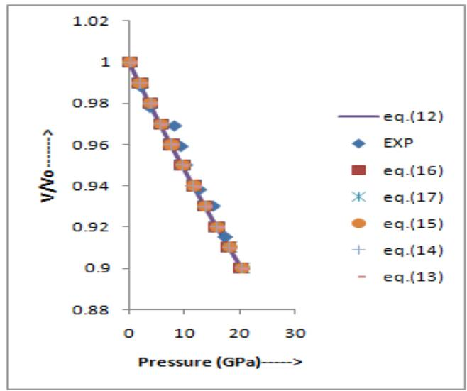
Figure 6: Pressure dependence of  $\frac{V}{V_0}$  for MgO
