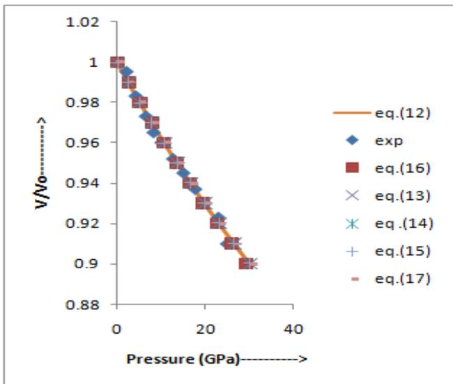
Figure 3: Pressure dependence of  $\frac{V}{V_0}$  for 3C-SiC (30 nm)
