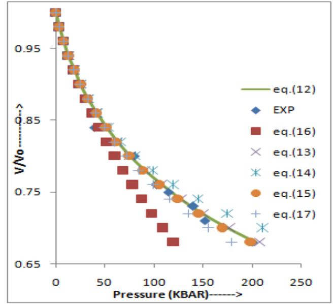
Figure 7: Pressure dependence of  $\frac{V}{V_0}$  for  $\text{C}_{60}$  solid
