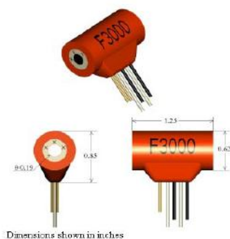
Figure 5: Frangibolt non-explosive release device.
