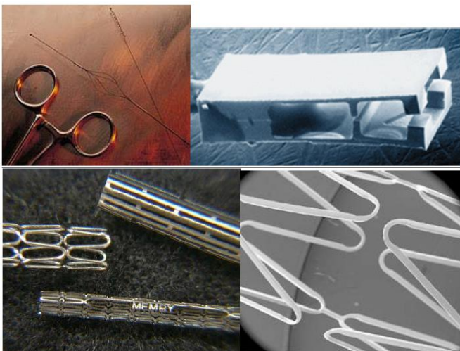
Figure 10: Surgical tools, microgripper and stents.
