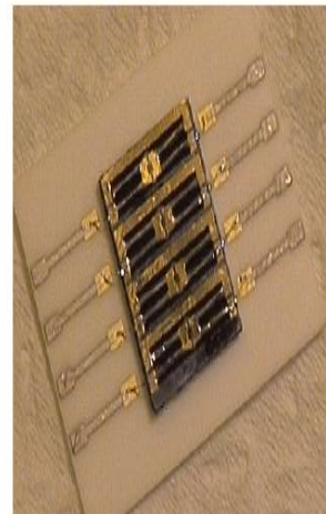
Figure 7: An array of four microvalves, the size of the array is 12.5 mm x 15 mm.
