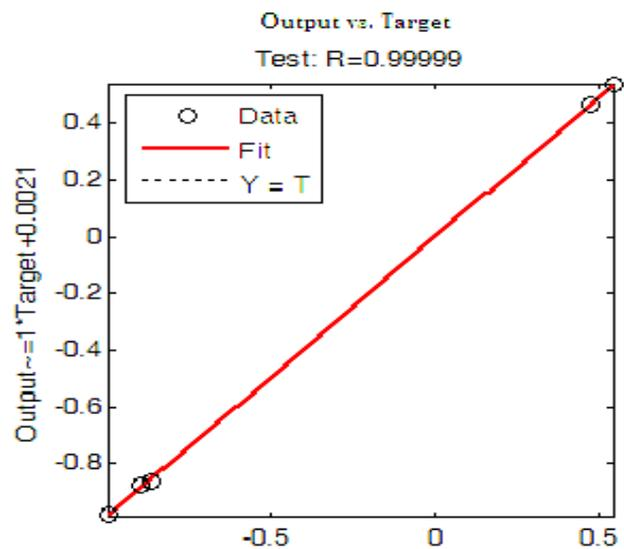
Fig. 4: Predicted Surface Roughness ( $R_a$ ) against the actual Surface Roughness
