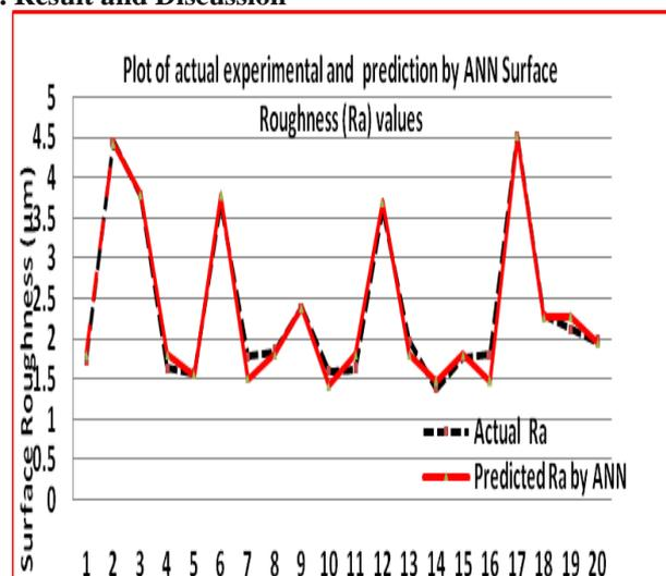
Fig. 5: Plot of actual experimental and prediction by ANN Surface Roughness ( $R_a$ ) values
