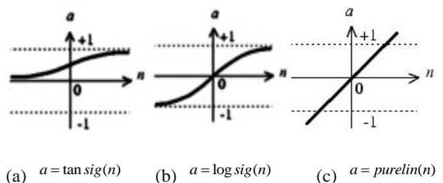
**Fig.2: Transfer functions used in hidden layer (a, b) & output layer (c)**
