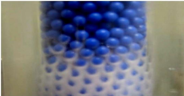
Fig.6. \text{CO}_2 ice formed at the packing surface during a capture cycle.
