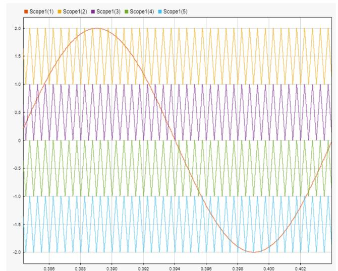
Fig 4.4 Level Shifted Sign PWM Generation
