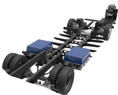
Fig.:- 04 – Battery packaging at chassis centre between front and rear axle
