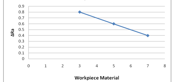
Fig. 15 Effect of the Workpiece material (B 4 C%) on \Delta R_a , at the magnetic flux density = 0.4T, concentration of abrasives = 55%, no. of cycles = 200, mesh number of abrasives = 150, extrusion pressure = 5 MPa.
