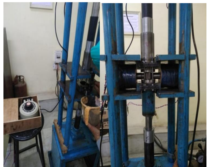
Fig. 3 Experimental Setup for Magnetic Abrasive Flow Machining (MAFM)
