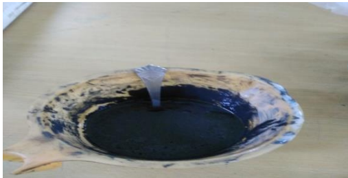
Fig. 5 Prepared abrasive putty
