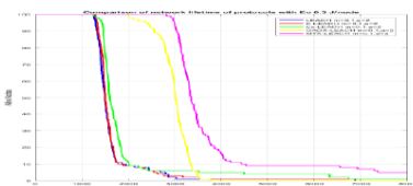
Figure 5: Network Lifetime Comparison of different protocols (at Initial energy E_0 = 0.3J/Node )
