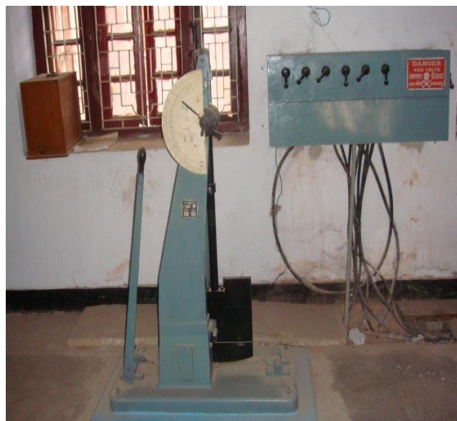
Fig. 2: Toughness (charpy impact) test
