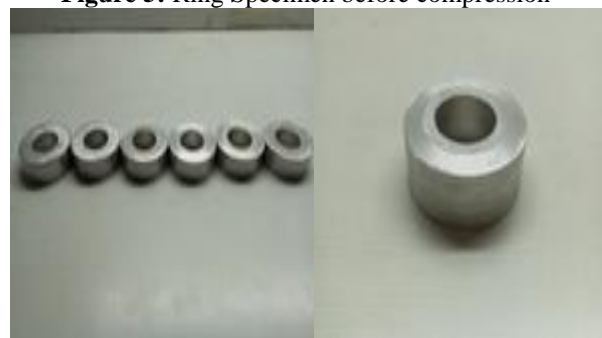
Figure 5: Ring Specimen before compression
