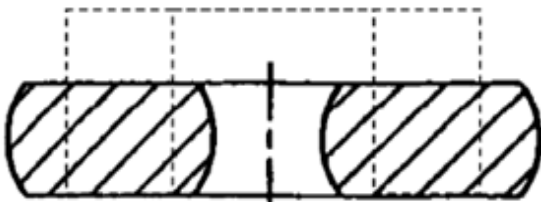
Figure 3: material flow under compression at high friction
