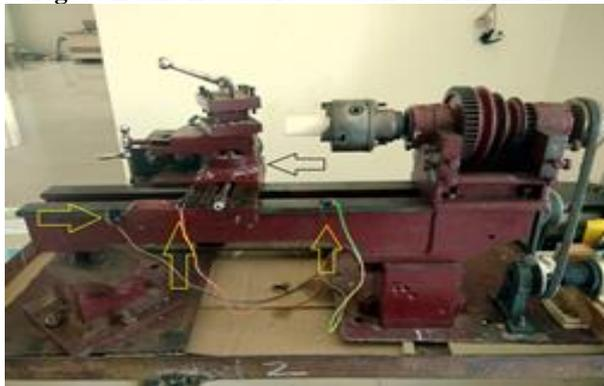
Fig. 8: Limit switches
