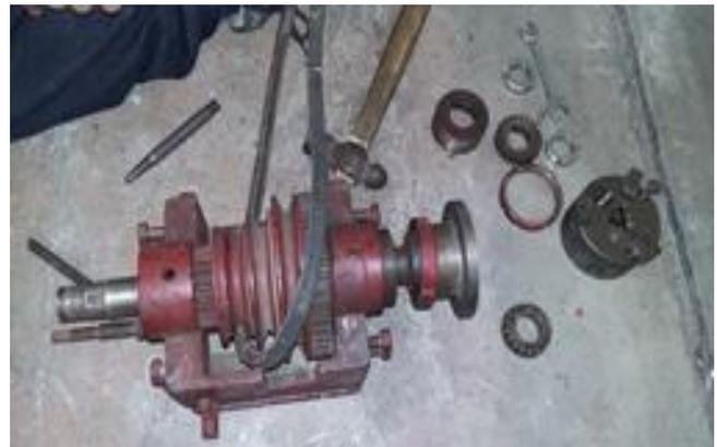
**Fig. 4: Removal of Head Stock Gearing Mechanism**
