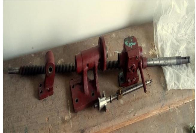
**Fig. 3: Lead Screw of X and Z axis**
