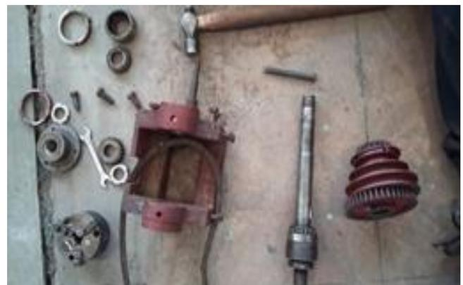
**Fig. 4: Removal of Head Stock Gearing Mechanism**
