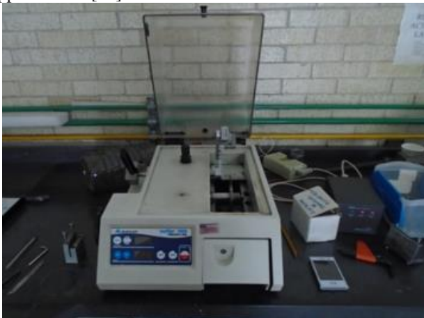
Fig. 2. Pre-cracked with Diamond Disk
