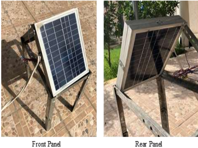
Figure (1). The double sided solar panel used in this study. The rear panel (right) was facing the ground when the front panel (left) is facing south.
