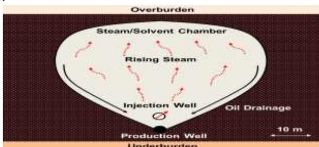
Fig. 1 Concept diagram of SAGD and solvent-SAGD process.
