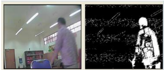
Fig. 2. Color image and background subtracted result image before filtering
