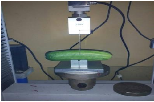
Figure 2: Cucumber fruit undergoing Warner Bratzler Test, using Universal Testing Machine (Testometric model, series 500-532)
