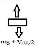
Now, from Newton's laws of motion we get,  $(mg + Vpg/2) = ma_1 \text{ where } a_1 \text{ is the downward acceleration.} \\ \Rightarrow a_1 = (mg + Vpg/2)/m$
