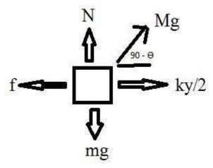
Here M is mass of the shield. According to figure of system description it will act at an angle  $\theta$  with the horizontal. So, we need to break the force in vertical and horizontal axis. Vertically upward force component = Mg\*cos $\theta$  Horizontally rightward force is Mg\*sin $\theta$  Now, equating the vertical force we get, N + Mg\*cos $\theta$  = mg
