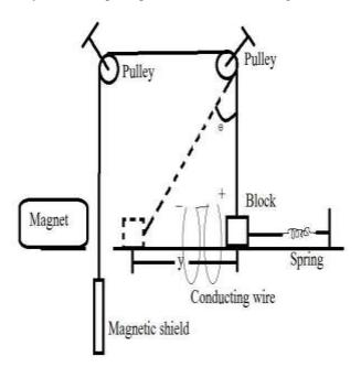
Here, the block is a magnet and the conducting wires are cut in the upper level to give the space for moving the magnet. Rest other are as indicated in the figure.
