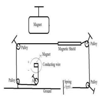
In the diagram above Pulley A's function is to maintain the magnet in one vertical line. Rest others are as shown in the diagram.
