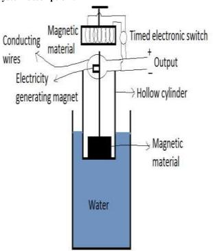
In the above figure everything is pointed out. The solid magnetic material is fastened with the hollow cylinder at its bottom. We will study the working principle in the next chapter.
