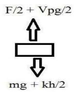
Now, from Newton's laws of motion, we get, (F/2 + Vpg/2) - (mg + kh/2) = ma $\Rightarrow a = [(F/2 + Vpg/2) - (mg + kh/2)]/m$
