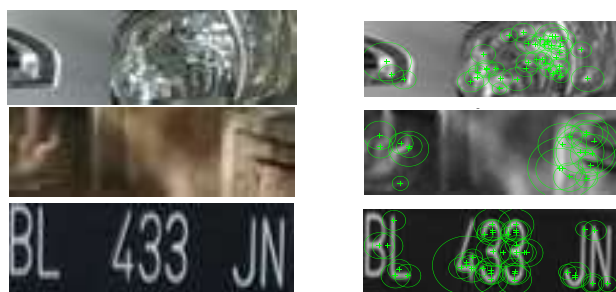
a) Detected plate candidates b) SURF keypoints
