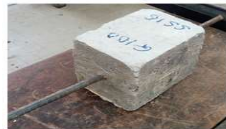
Pull-out test specimen
