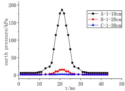
Figure 10. The influence range at the depth of 10cm, 20cm and 30cm by 7.5N.m tamping energy
