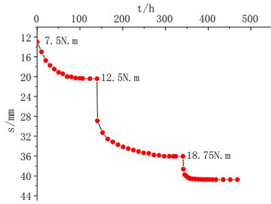
Figure 6. Curves of settlement with time at the top of soft soil under dynamic consolidation
