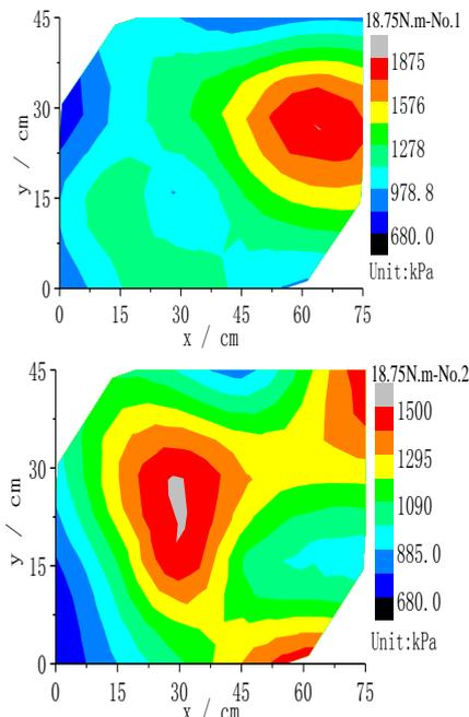
Figure 5. the soil body resistance nephogram when ramming energy is 18.75N·m
