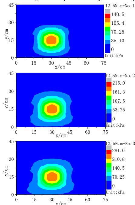
Figure 12. Influence range at the depth of 10cm by 12.5N-m tamping energy
