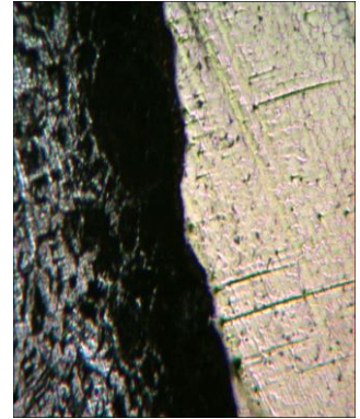
Figure 4: fusion boundary on 200 X magnification
