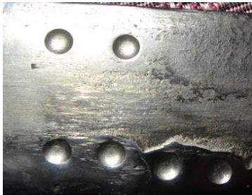
figure 2: hardness tested work piece
