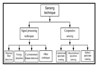
Figure 2 Classification of Spectrum Sensing Techniques
