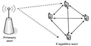
Figure 9 Decentralized Cooperative Spectrum Sensing
