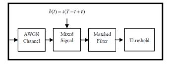
Figure 3 Block Diagram of Matched filter detection
