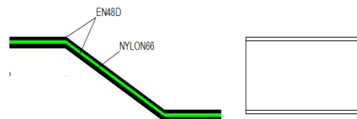
composite leaf spring : Material EN304 + Nylon-66
