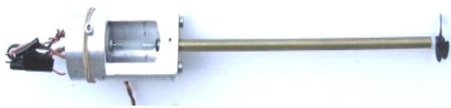
Motor and propeller mounted in holder.
