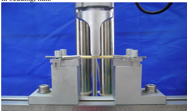
Fig 1 A test equipment for measurement of bending properties of millet stems.
