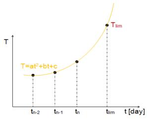
$$\begin{split} t_{pred} &= t_{lim} - t_3 \\ t_{lim} &= \min(-\frac{b}{2a} \pm \frac{\sqrt{D}}{2a}) \\ D &= b^2 - 4a(c - T_{lim}) \\ T_{lim} &\geq c - \frac{b^2}{4a} \end{split}$$
