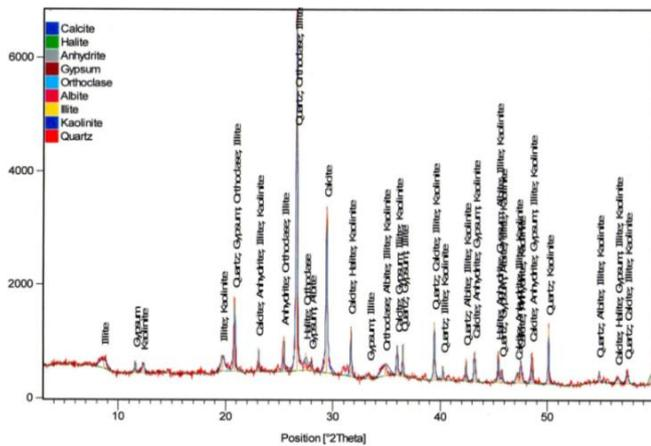
Fig.1. Mineralogical analysis of bricks in earth of the walls of the ksour
