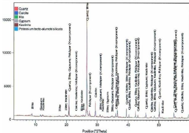
Fig.2. Mineralogical Analysis of the mortar of jointement
