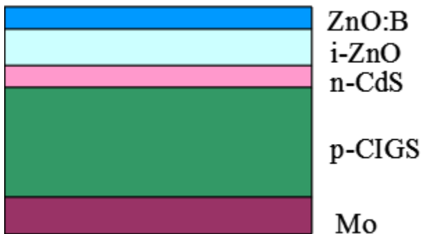
Fig. 1: Structure of a CIGS device
