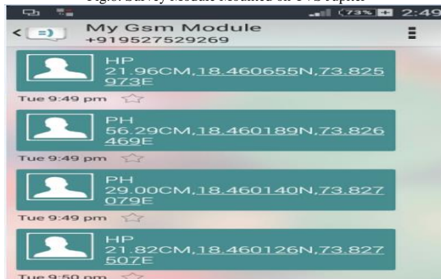
Fig.9: Real Time Readings Taken by the survey module
