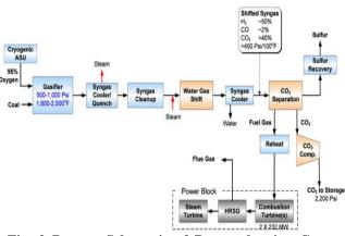
Fig. 2 Process Schematic of Pre-combustion Capture [10]
