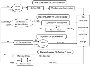
Fig. 1 CO<sub>2</sub> Capture technologies [1]
