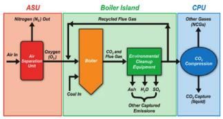
Fig. 3 Oxyfuel combustion [11]
