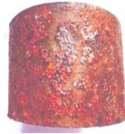
Figure 2 EN9/070M55 steel components after 72 hours
