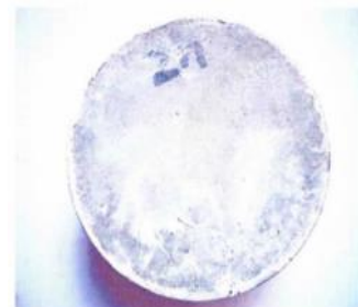
Figure 4 Zinc coated components after 72 hours.
