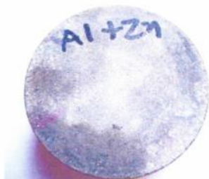
Figure 5 Zn-Al coated Components after 72 hours.
