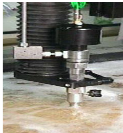
Fig. 1 Abrasive water jet machining cutting head
