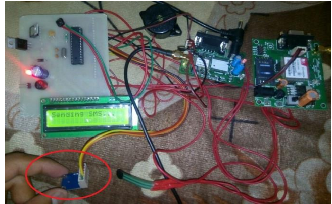
Figure 8: When the car takes a tilt(accelerometer is tilted beyond the prescribed safe limit)
