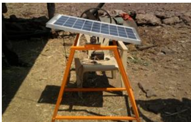
Fig.12. Solar tracking system
