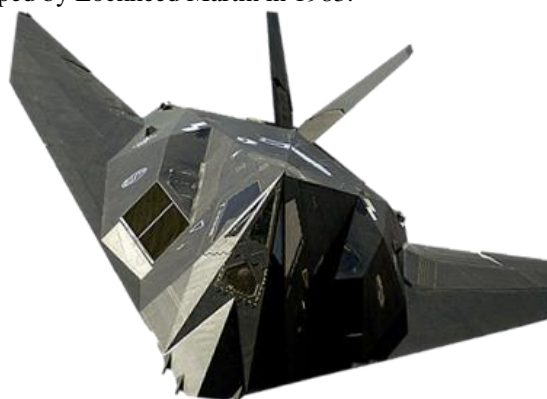
Figure 1: The F-117A Nighthawk Stealth Fighter, a single seat, twin engine aircraft developed by Lockheed Martin.
