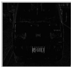
Fig. 2.2: Image edge use Sobel method.
