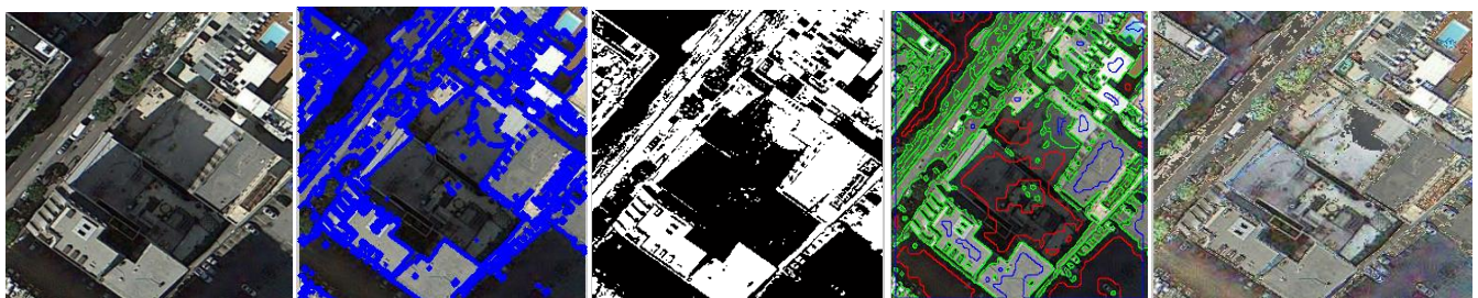
Fig.4.Examples of shadow detection and removal using SVM classifier. (a) QuickBird image. (b) Segmentation result of (a). (c) Threshold shadow detection result after segmentation. (d)IOOPL generated (e) Reconstructed image
