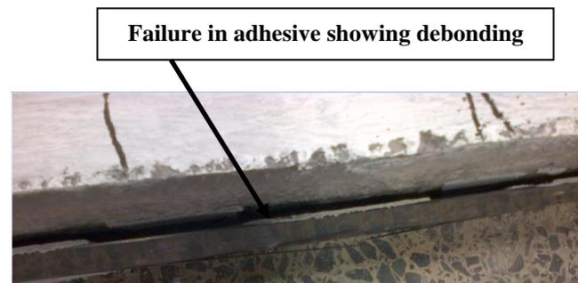
Figure 13. Intermediate crack induced debonding (b)
