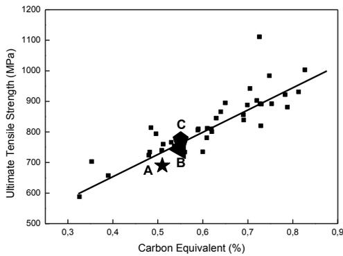
Figure 2. Influence of carbon equivalent on the ultimate tensile strength. A, B and C weld metals of the present work in comparison with other authors [15],[19],[20],[22]-[29].
