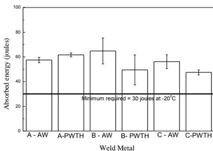
Figure 3. Results of Charpy-V impact tests.
