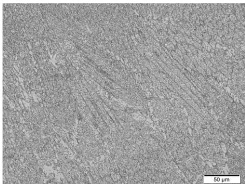
Figure 8. Occurrence of segregation associated with M-A constituents. Etching: Nital 2%.
