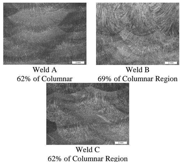
Figure 5. Optical micrographs (OM) of the region from where specimens for mechanical testing were sampled.
