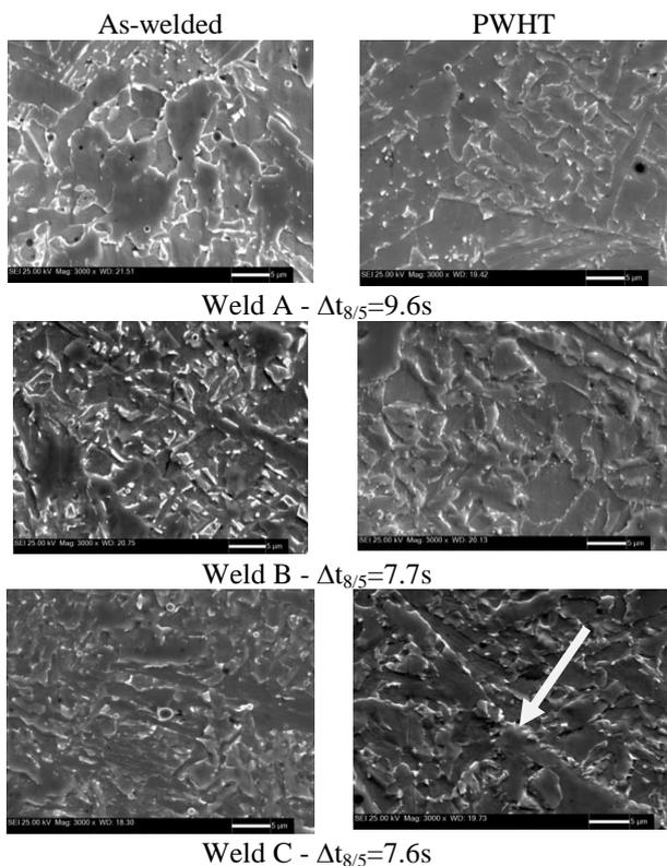
Figure 7. Weld metal microstructures of the regions correspondent to the position of the Charpy-V notch. Etching: nital 2%.
