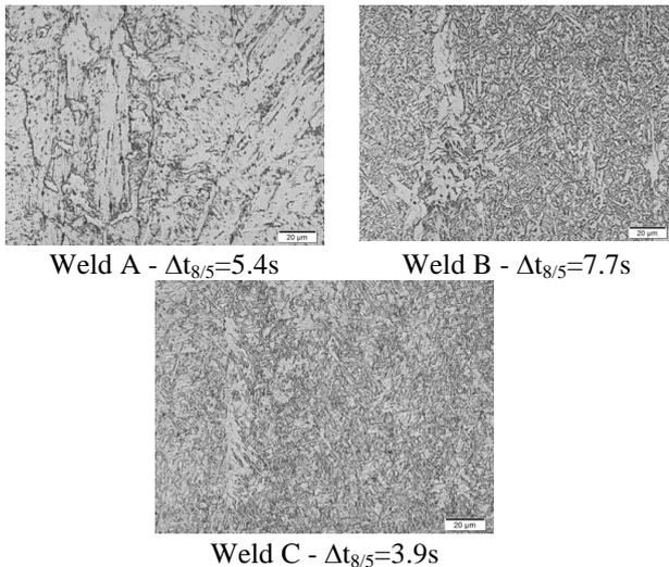
Figure 6. Top bead microstructures of the weld metals observed by Optical Microscopy (OM).
