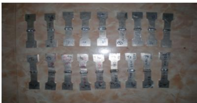
Fig 2: Test specimens after welding
