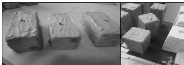
FIG. 05, application of the mixture of the brick blocks as coating
