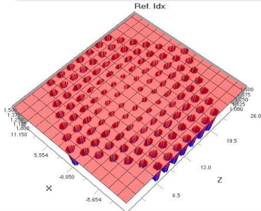
Fig. 6 Cross section of proposed PCF at pitch=2.05µm
