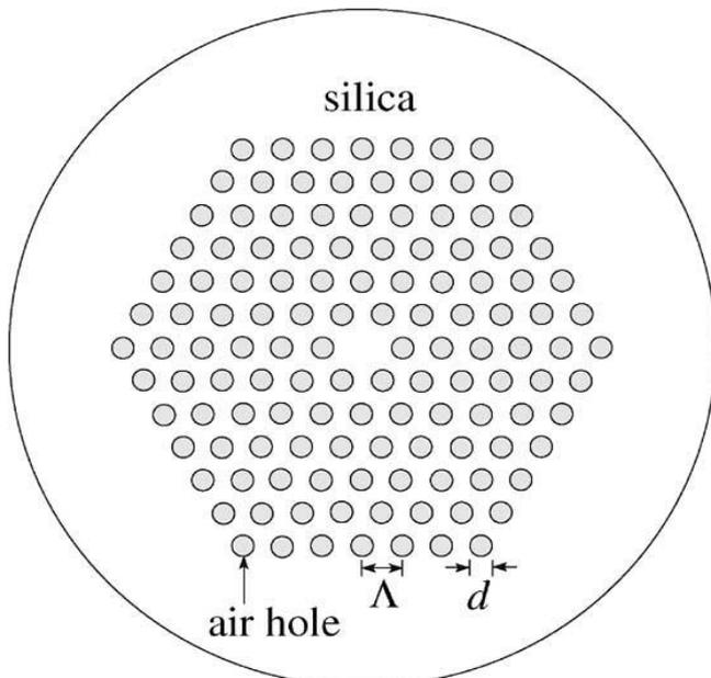
Fig.2 Photonic crystal fiber representation
