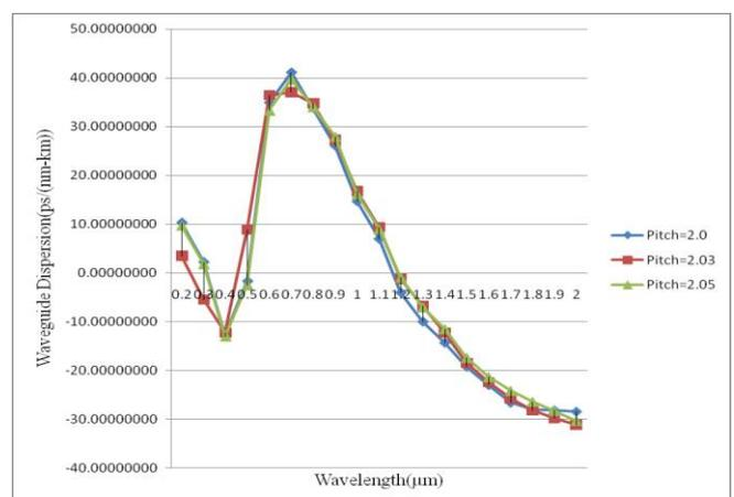
Fig. 8 Waveguide dispersion with wavelength
