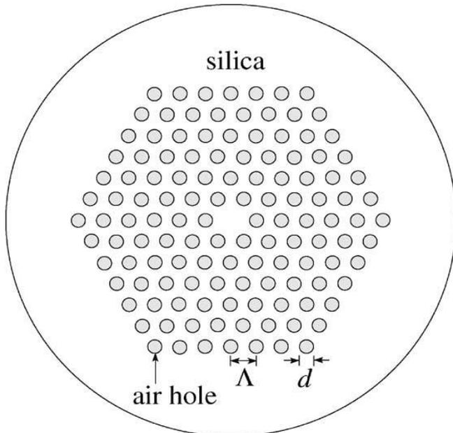
Fig.2 Photonic crystal fiber representation
