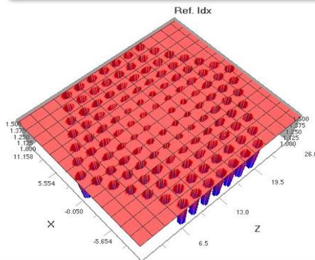
**Fig. 5 Cross section of proposed PCF at pitch=2.03μm**
