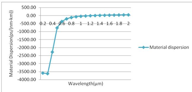
**Fig. 3 Material Dispersion of Fused Silica Glass**
