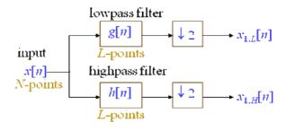
Fig.4. The block diagram of the 1-D DWT
