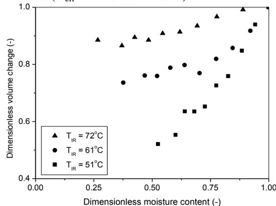
Fig. 5: Dimensionless volume change ( $V_p/V_{p0}$ ) of the particles as a function of dimensionless moisture content (XR) during IR drying at different temperatures.
