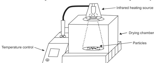
Fig. 1: Schematic diagram of the IR dryer.
