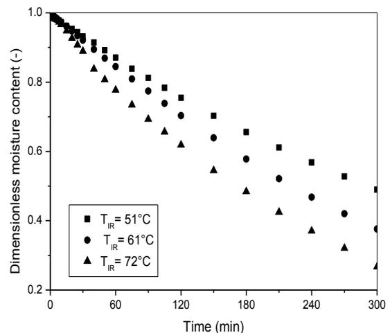
Fig. 2: Dimensionless moisture content as a function of time during IR drying at different temperatures.
