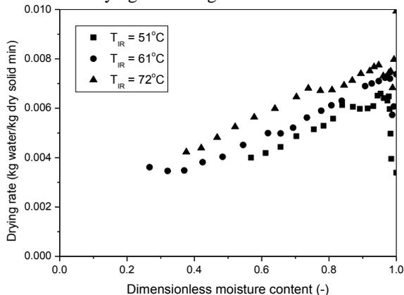
Fig. 4: Drying rate as a function of dimensionless moisture content during IR drying at different temperatures.
