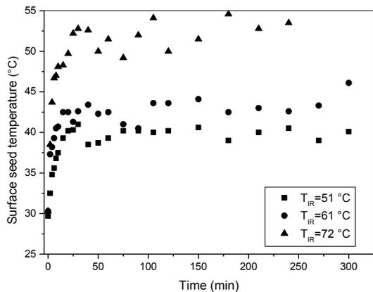
Fig. 3: Surface seed temperature as a function of time during IR drying at different temperatures.
