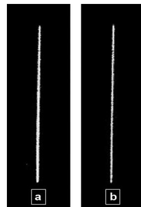
Fig 5.Slit images for (a) energy integrating mode and (b) single photon counting mode[3].
