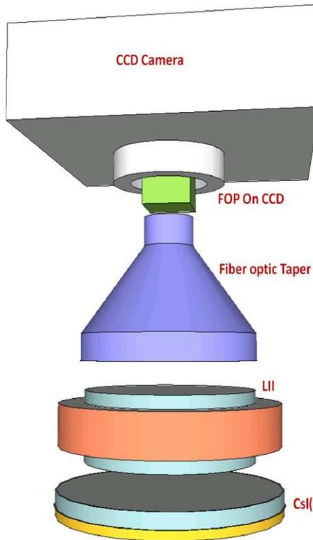
Fig. 2. Schematic diagram of MAF
