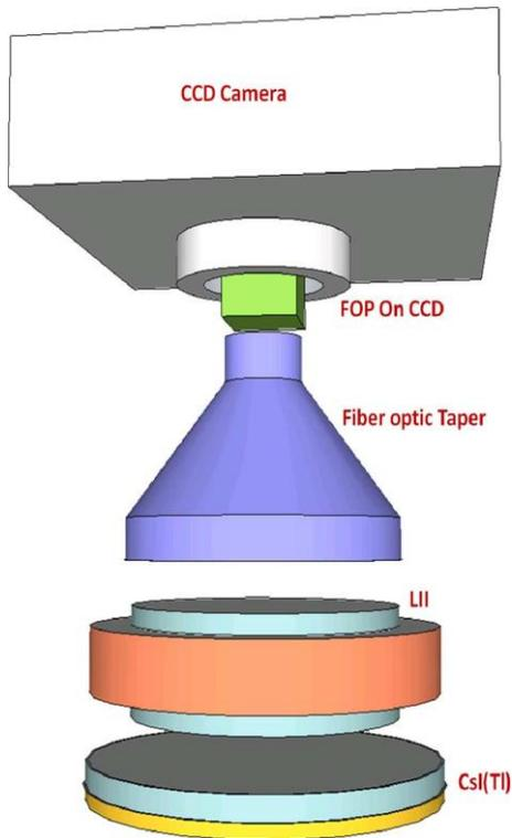
Fig. 2. Schematic diagram of MAF
