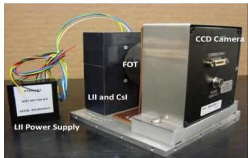
Fig 3. Micro angiographic Fluoroscope[3].
