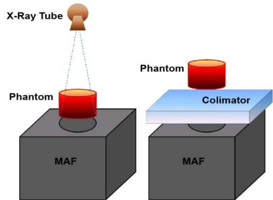
Fig 4. Experimental set up diagram for (left) X-ray Imaging and (right) Radionuclide Imaging[3].
