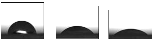
Fig. 9. Water drop shape changes of the acetic anhydride modified sample surface
