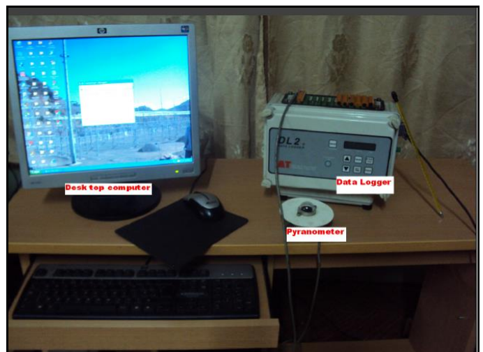
Fig 2. Pictorial representations of DL2e Data Logger and pyranometer
