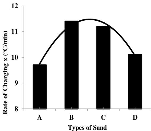
Fig. 6 Rate of Charging Some Types of Sand.
