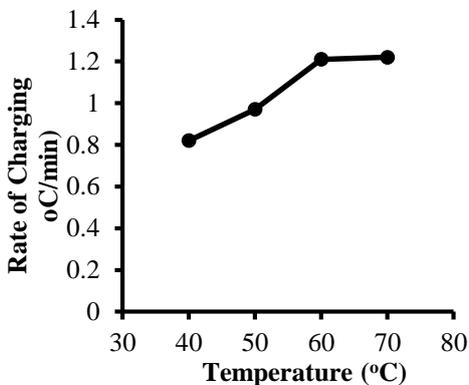
Fig. 3 Rate of Charging Sands at Different Temperatures
