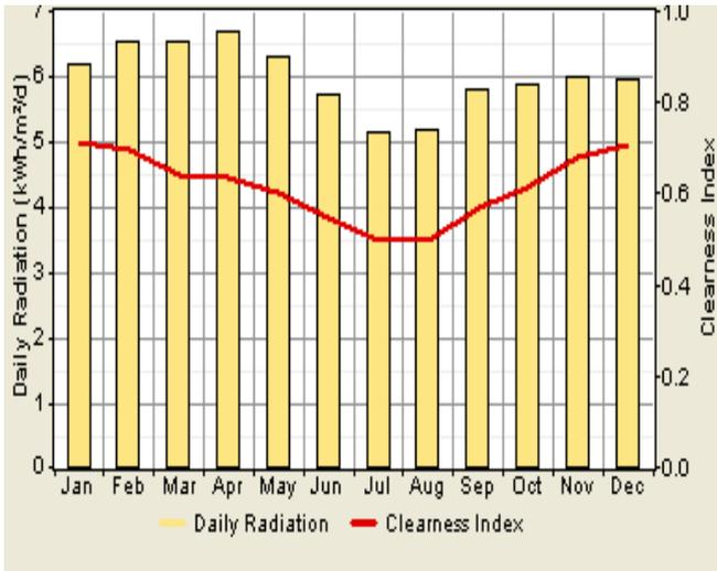
Figure 4 Global Horizontal Radiation and Clearness Index
