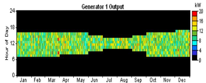
**Figure 15** Generator Output During Sunshine Hours
